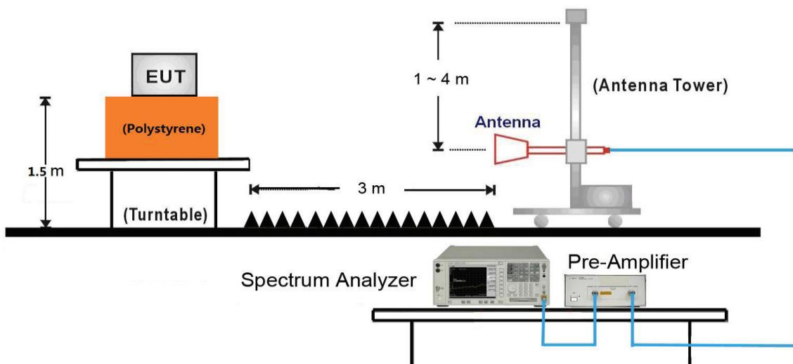
18GHz ~25GHz Test Setup:
