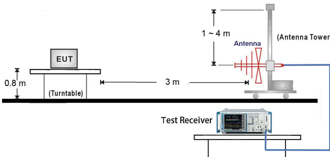
1GHz ~ 18GHz Test Setup:
