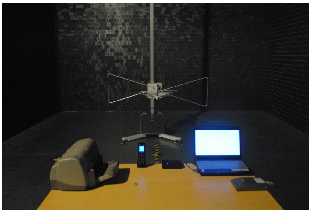
Radiated Emission test view (Frequency above 1GHz)
