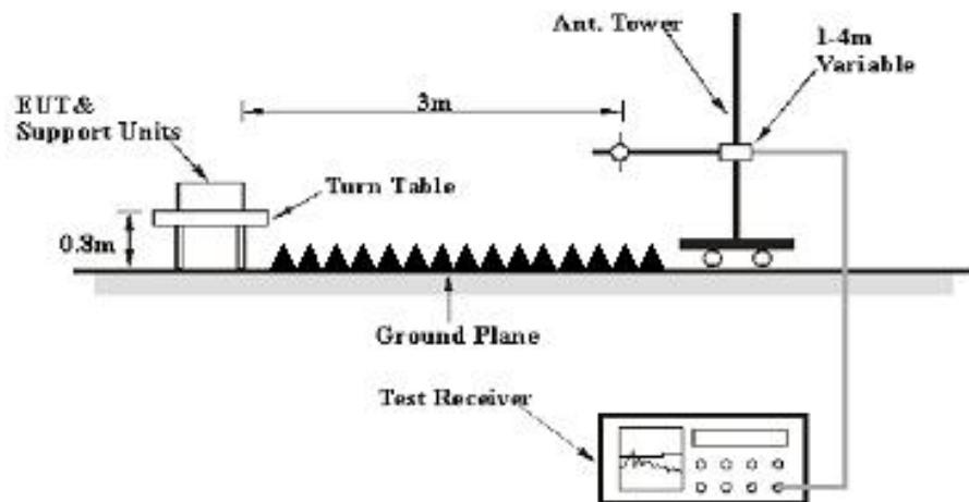
The radiated emissions were performed in the 3 meters chamber test site, using the setup accordance with the ANSI C63.4-2014. The specification used was with the FCC Part 15 B Class B limits.
