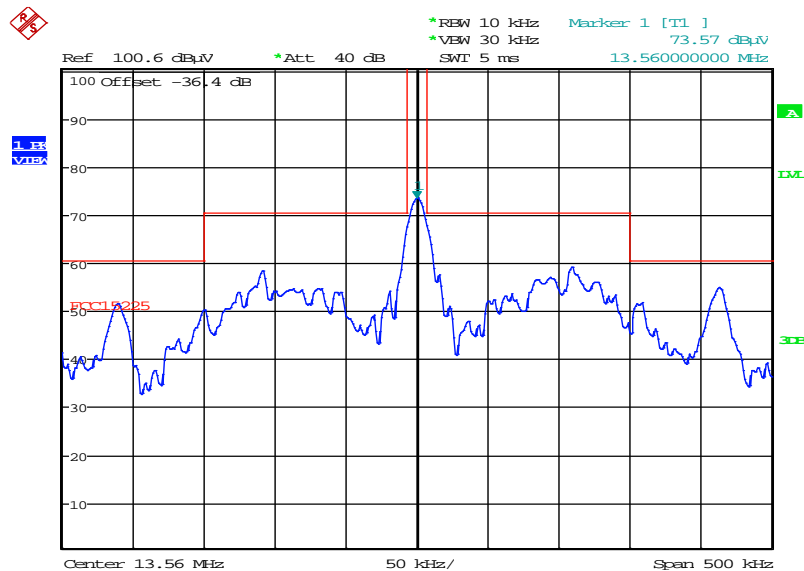
Plot 3: Spectrum mask zoomed (the limits are recalculated according to the ANSI C63.10-2013 sub clause 6.4)
