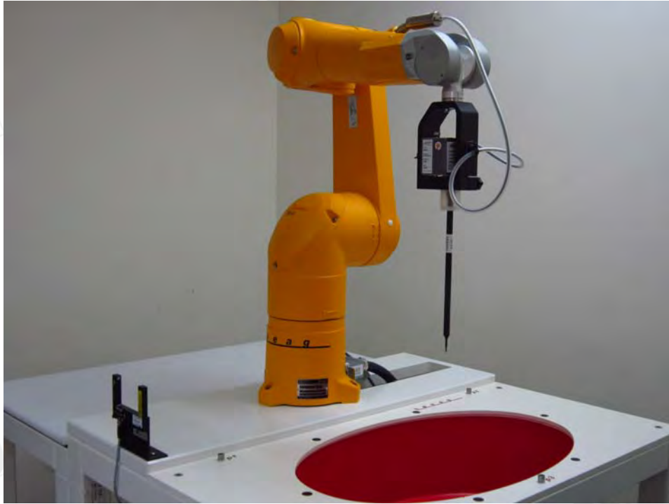
Fig.1 Photograph of the SAR measurement system
