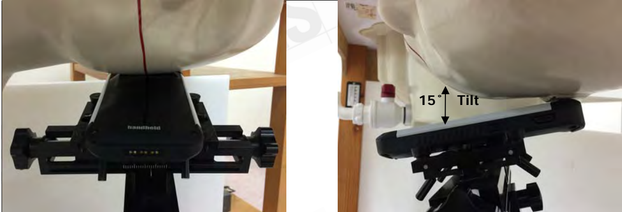
Fig.6 Left Head Section / Ear-Tilt Position(15°)
