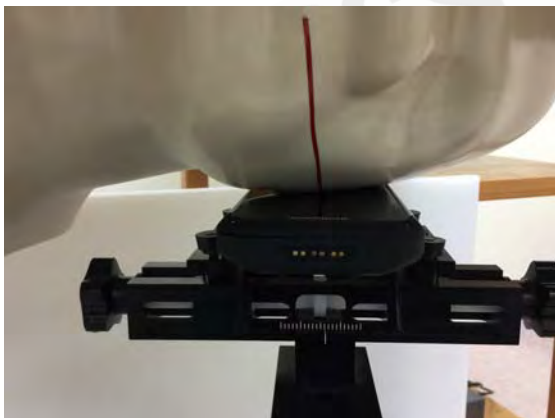
Fig.5 Left Head Section / Cheek-Touch Position
