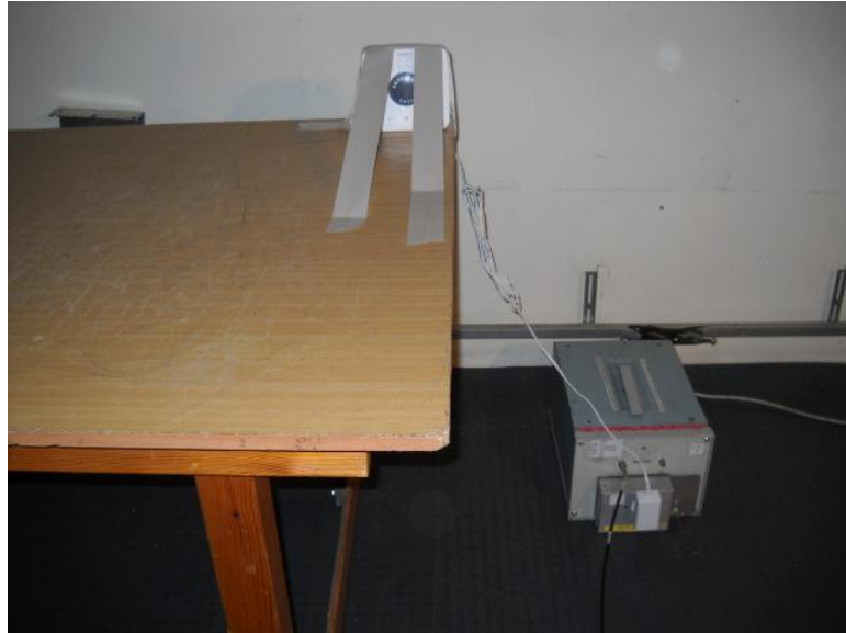
Photograph 8.1.2 Setup for conducted emission measurements
