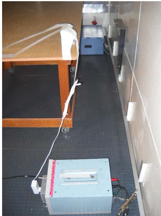
Photograph 8.1.2 Setup for conducted emission measurements
