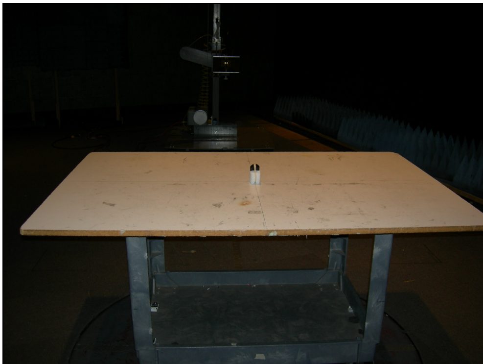
Figure 4: Radiated Emissions Test Setup – Y-POS – Back View
