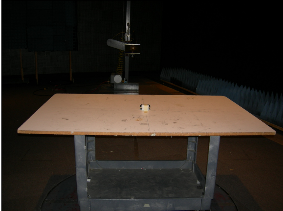
Figure 6: Radiated Emissions Test Setup – Z-POS – Back View
