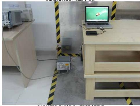
RADIATED EMISSION TEST SETUP
