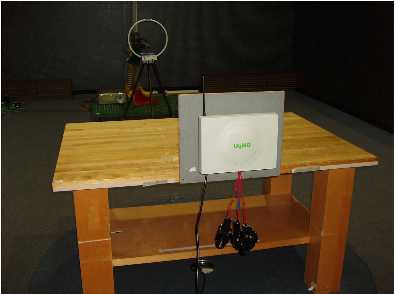
Photo 4 – Rear View of the Radiated Emissions Test Set-up with the Loop Antenna
