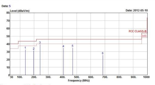
Site : 966 Chamber 5 Condition : FCC CLASS-B 3m ANT\_30M~1G\_LF HORIZONTAL
