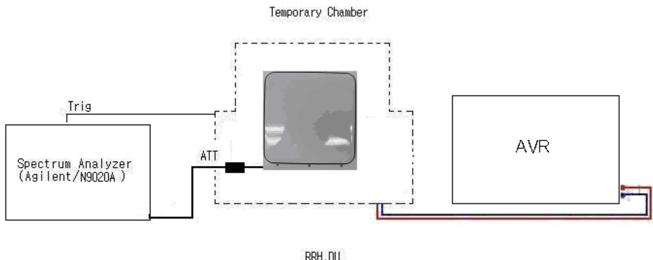
According to FCC §2.1046 (c), for transmitters other than single sideband, independent sideband and controlled carrier radiotelephone, power output shall be measured at the RF output terminals when the transmitter is adjusted in accordance with the tune-up procedure to give the values of current and voltage on the circuit elements specified in § 2.1033(c). The electrical characteristics of the radio frequency load attached to the output terminals when this test is made shall be stated.
