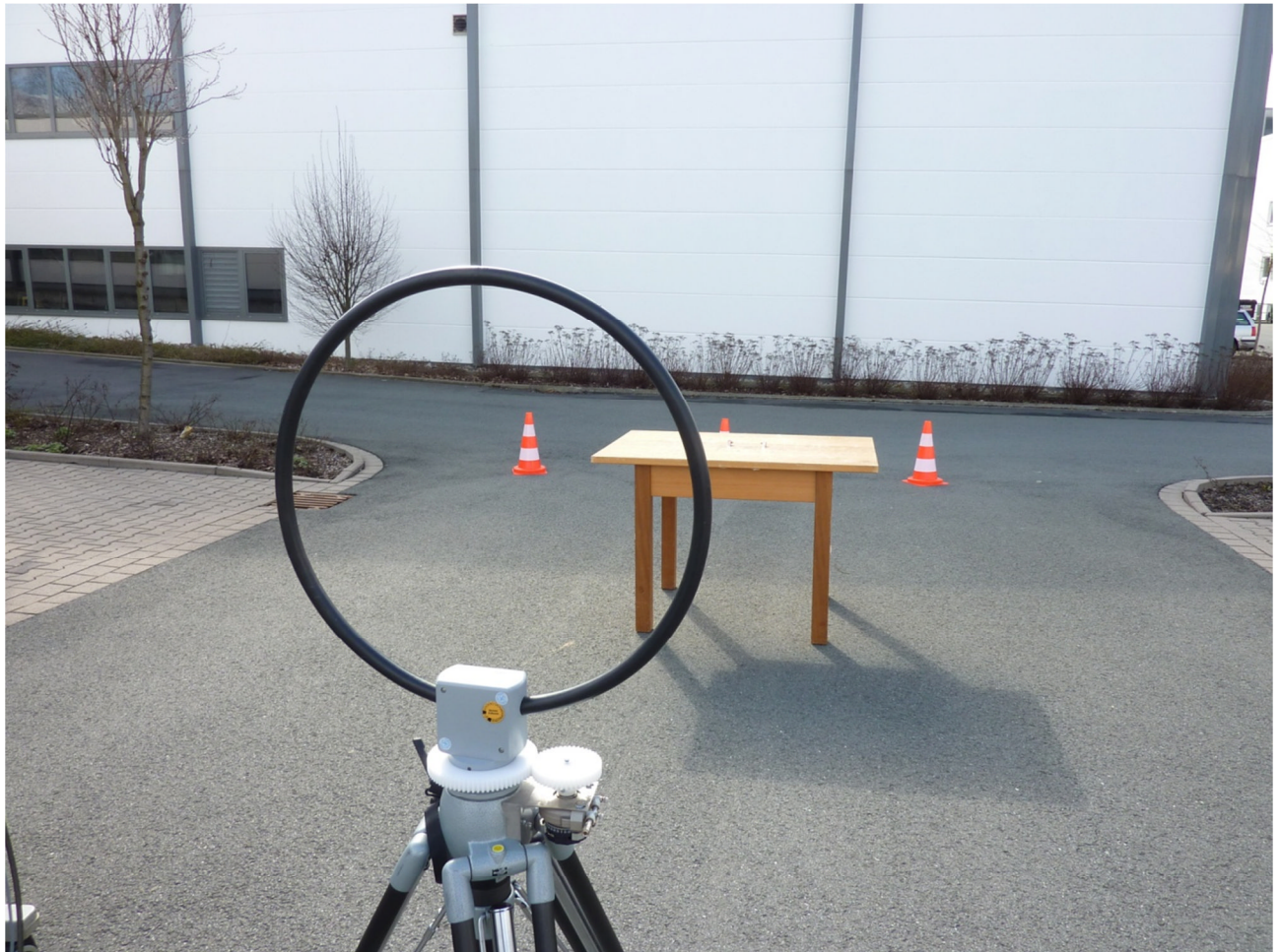
120962emi3.JPG: Test set-up final radiated emission (H-Field)
