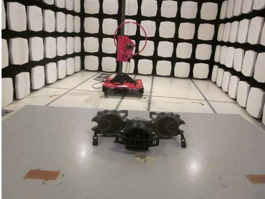
Measurement of Radiated Emission Test Set Up
