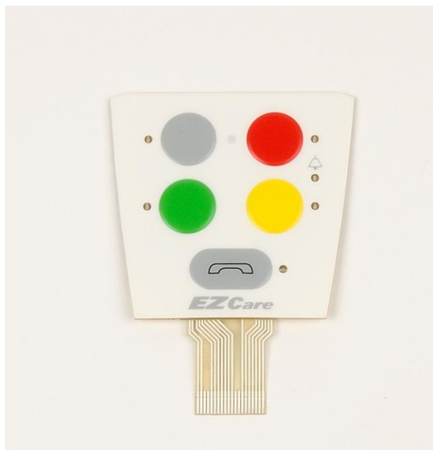
Picture 7: Front view of keyboard (red button version) with RFID antenna foil
