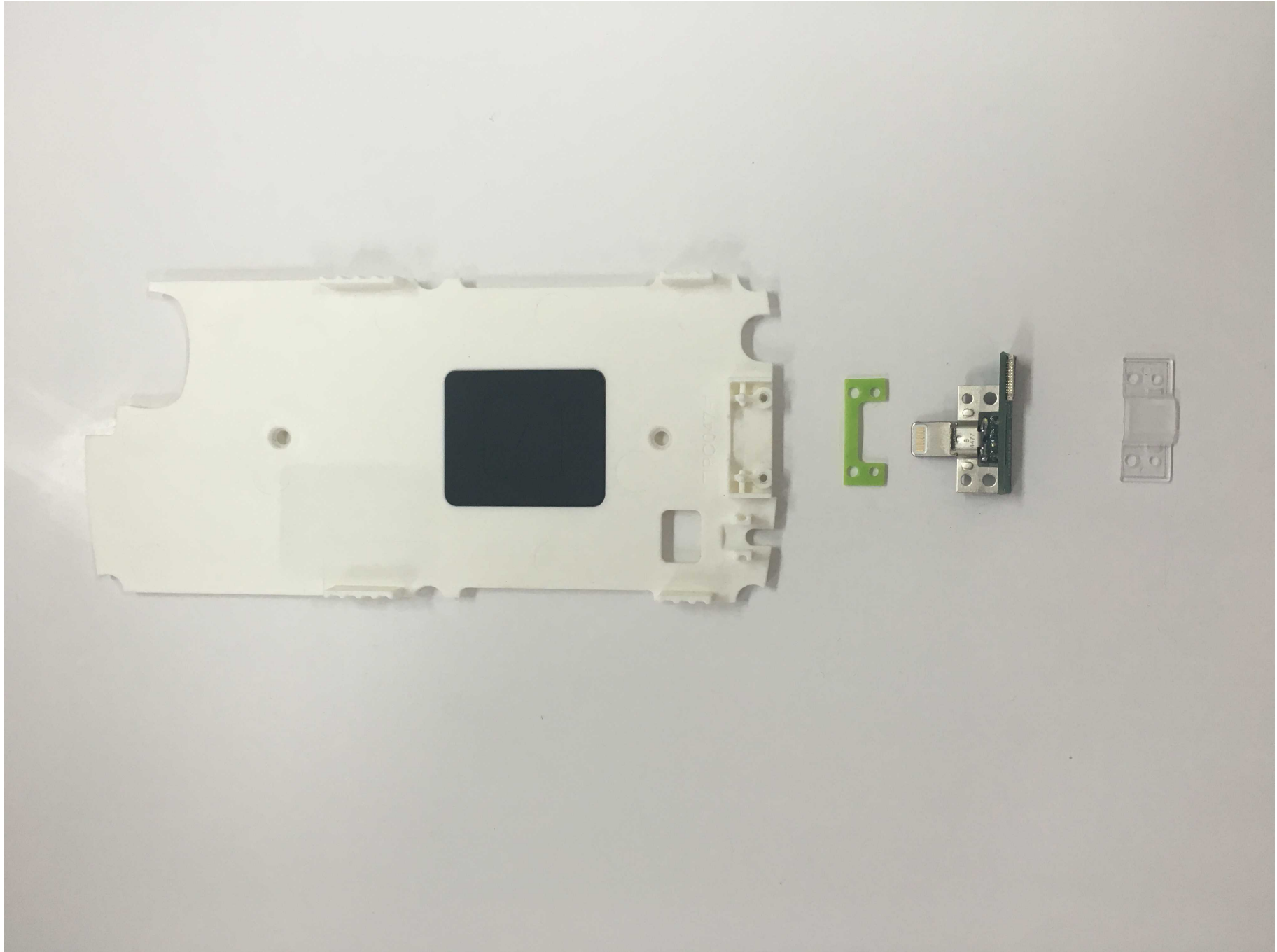
InfiniaX - carrier and disassembled Apple 9-pin lightning connector, PCB C019002
