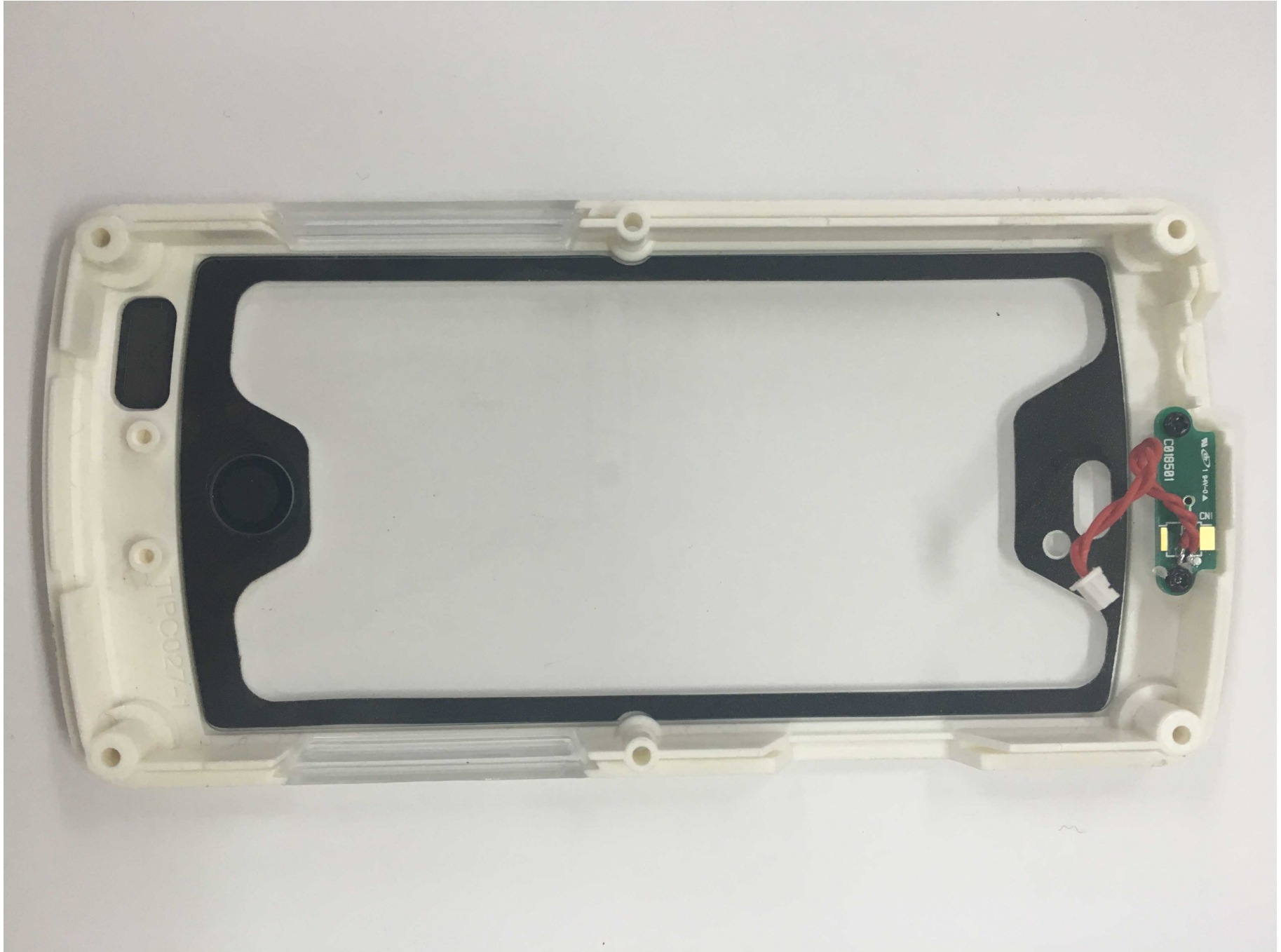
Infineax – upper enclosure back view, front speaker PCB C018501
