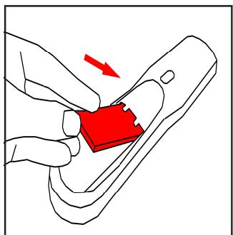
Push down on the back of the battery to clip it in place. Replace the cover.
