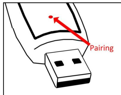
Place the USB Dongle in pairing mode. This is done by slotting the USB Dongle into the Media Center and then pushing and holding the pairing button on the USB dongle, until it starts to flash rapidly. At this point remove the paper clip. The USB Dongle is now ready to receive the pairing request from the Voice Remote.
