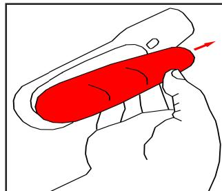
The battery cover falls downwards and can then be removed.
