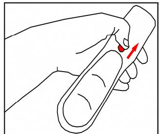
Hold the remote with the battery cover facing down. Slide the release clip towards the top to release the cover.
