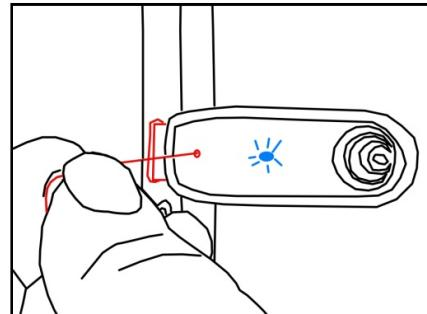
To get the Voice Remote to issue the pairing request you must push the pairing button on the remote until the light on the USB goes solid. At this point the USB dongle and Voice Remote have been paired.
