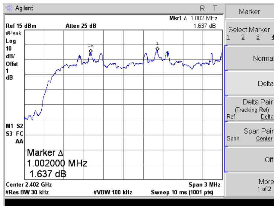
Channel Spacing (Middle CH=1MHz)
