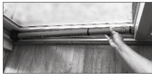
Adjust the length to fit the sliding door or window track using the push button. Repeat steps above on how to adjust the bar length. Leave some space to easily remove the security bar.
