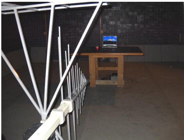
Photograph No.1 Setup for radiated emission measurements in 30 – 1000 MHz in the anechoic chamber
