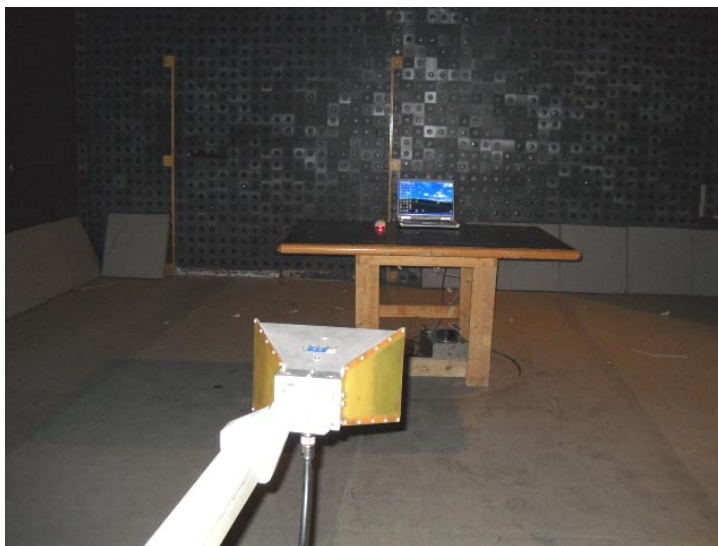
Photograph No.2 Setup for radiated emission measurements above 1 GHz in the anechoic chamber
