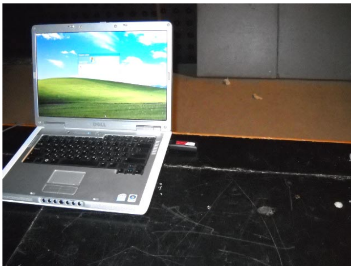
Photograph No.3 Setup for radiated emission measurements in the anechoic chamber, EUT close view
