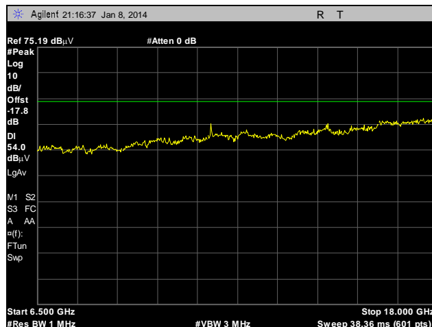
Plot 117. Radiated Spurious Emissions, Internal Antenna, 802.11n 20 MHz, 5745 MHz, 6.5 GHz – 18 GHz, Peak under Average
