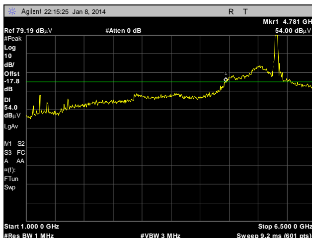
Plot 146. Radiated Spurious Emissions, External Antenna, 802.11n 20 MHz, 5745 MHz, 1 GHz – 6.5 GHz, Peak under Average
