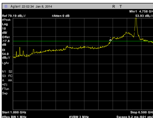
Plot 133. Radiated Spurious Emissions, External Antenna, 802.11a, 5745 MHz, 1 GHz – 6.5 GHz, Peak under Average
