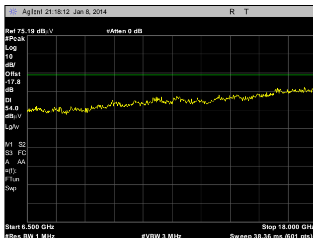
Plot 127. Radiated Spurious Emissions, Internal Antenna, 802.11n 40 MHz, 5755 MHz, 6.5 GHz – 18 GHz, Peak under Average
