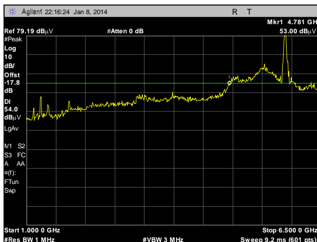
Plot 155. Radiated Spurious Emissions, External Antenna, 802.11n 20 MHz, 5825 MHz, 1 GHz – 6.5 GHz, Peak under Average
