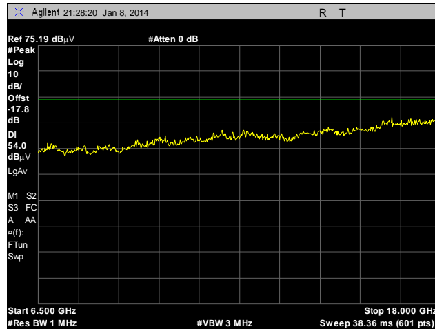
Plot 165. Radiated Spurious Emissions, External Antenna, 802.11n 40 MHz, 5795 MHz, 6.5 GHz – 18 GHz, Peak under Average
