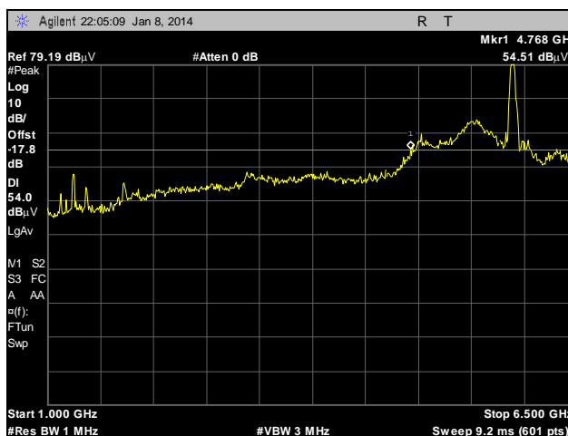
Plot 142. Radiated Spurious Emissions, External Antenna, 802.11a, 5825 MHz, 1 GHz – 6.5 GHz, Peak under Average
