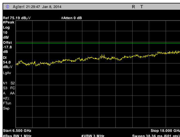
Plot 139. Radiated Spurious Emissions, External Antenna, 802.11a, 5785 MHz, 6.5 GHz – 18 GHz, Peak under Average
