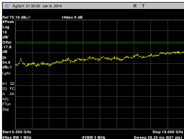
Plot 157. Radiated Spurious Emissions, External Antenna, 802.11n 20 MHz, 5825 MHz, 6.5 GHz – 18 GHz, Peak under Average
