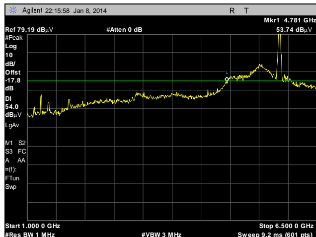
Plot 150. Radiated Spurious Emissions, External Antenna, 802.11n 20 MHz, 5785 MHz, 1 GHz – 6.5 GHz, Peak under Average
