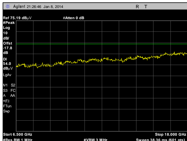
Plot 161. Radiated Spurious Emissions, External Antenna, 802.11n 40 MHz, 5755 MHz, 6.5 GHz – 18 GHz, Peak under Average
