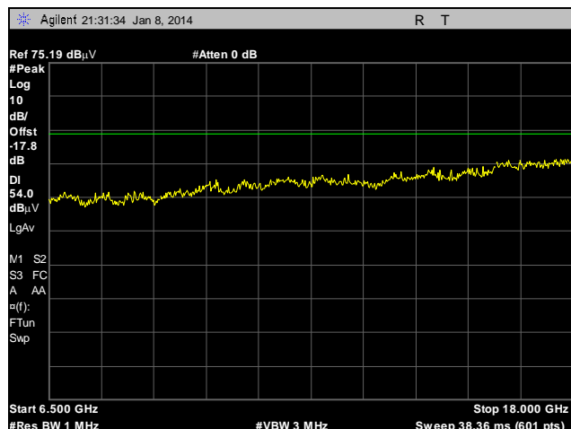
Plot 152. Radiated Spurious Emissions, External Antenna, 802.11n 20 MHz, 5785 MHz, 6.5 GHz – 18 GHz, Peak under Average
