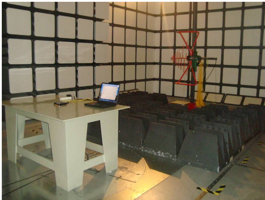
Below 1 GHz: Spurious Radiated Emissions - Rear View
