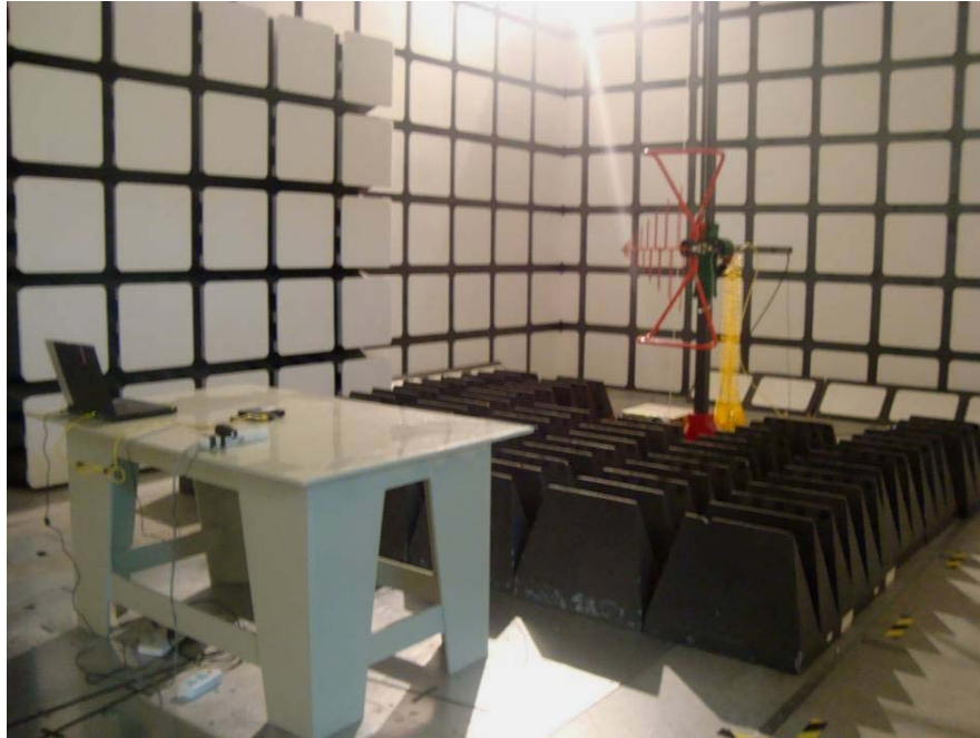
Below 1 GHz: Spurious Radiated Emissions - Rear View
