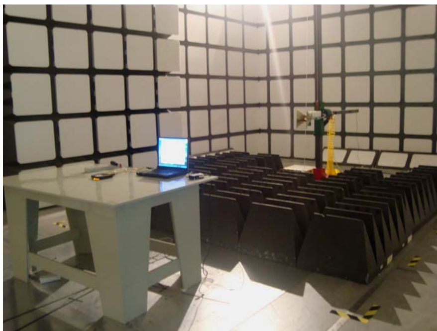
Above 1 GHz: Spurious Radiated Emissions - Rear View
