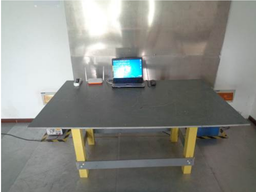
Conducted Emissions Test Setup Front View
