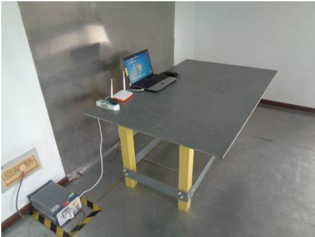
Conducted Emissions Test Setup Side View
