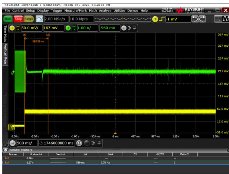
Figure 24 - Switching Time (Simplex), +55.0 °C, 31.2 V DC
