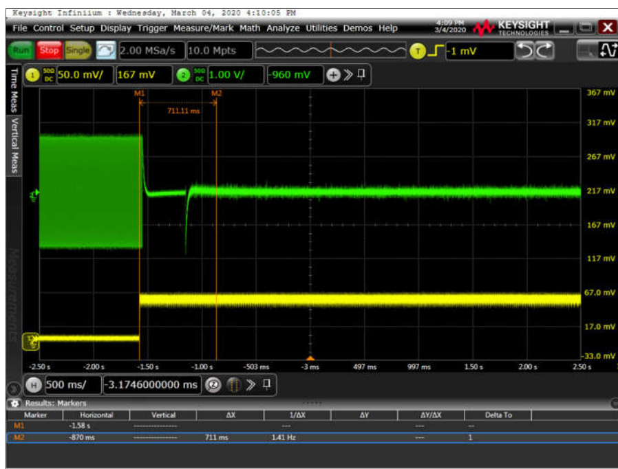
Figure 23 - Switching Time (Simplex), +55.0 °C, 10.8 V DC
