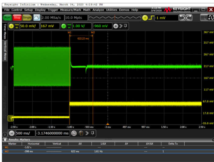
Figure 28 - Switching Time (Duplex), +55.0 °C, 10.8 V DC
