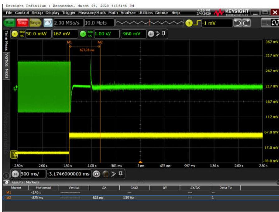
Figure 29 - Switching Time (Duplex), +55.0 °C, 31.2 V DC
