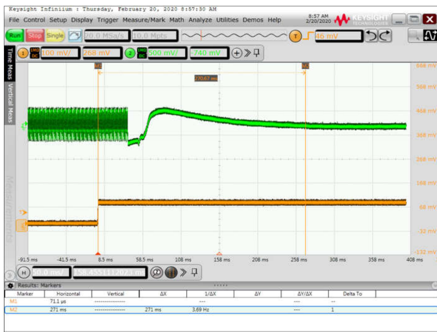
Figure 27 - Switching Time (Duplex), -15.0 °C, 31.2 V DC
