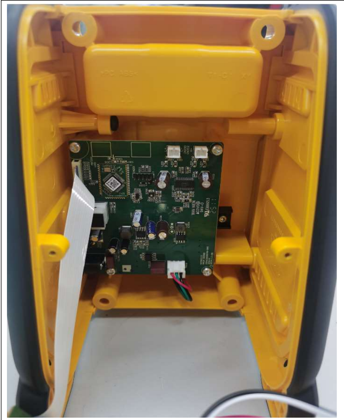
Rear Enclosure Internal – Main PCA mounting
