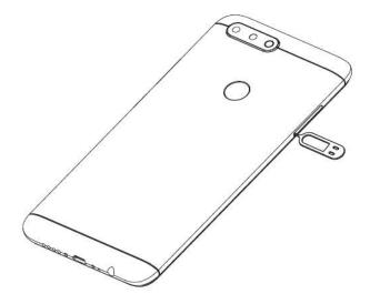
2) Put SIM cards and SD card to card tray correctly.
