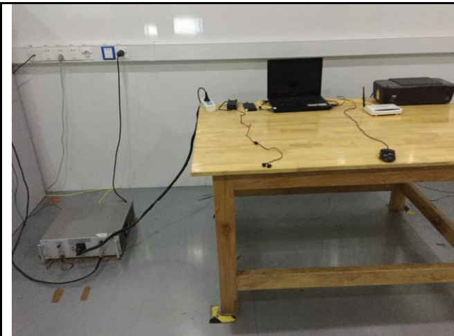
Conducted Emissions Test Setup – Front View
