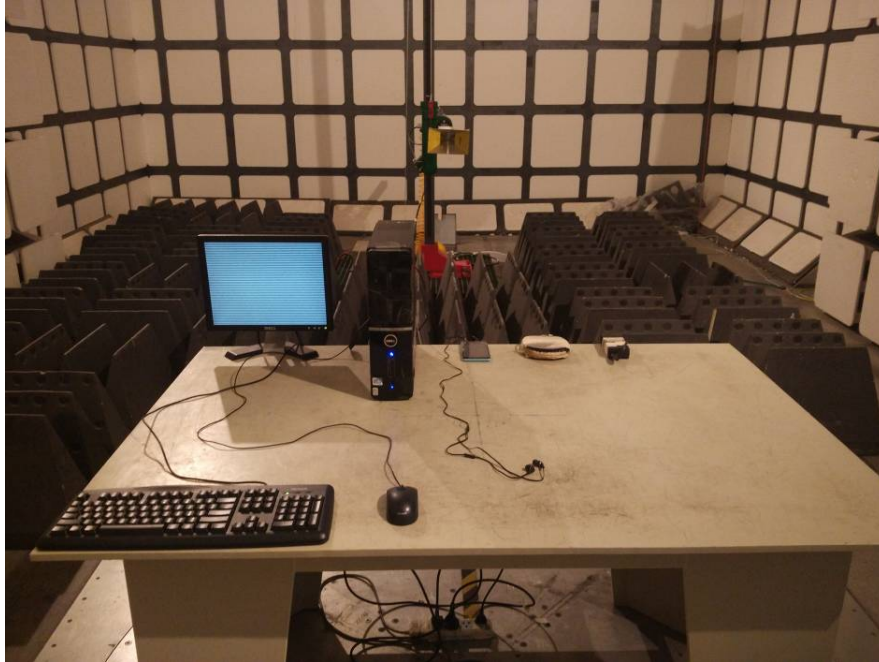
Radiated Emissions – Front View (Above 1 GHz)
