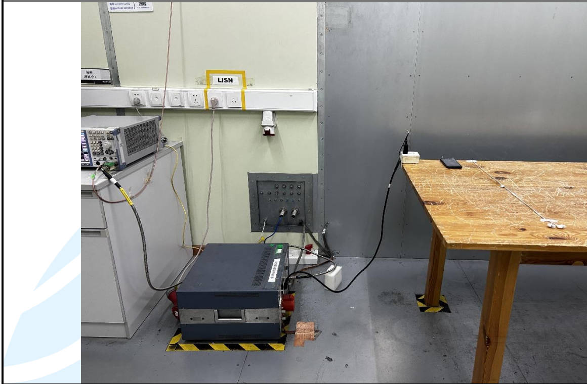
Conducted Emission Test Setup
