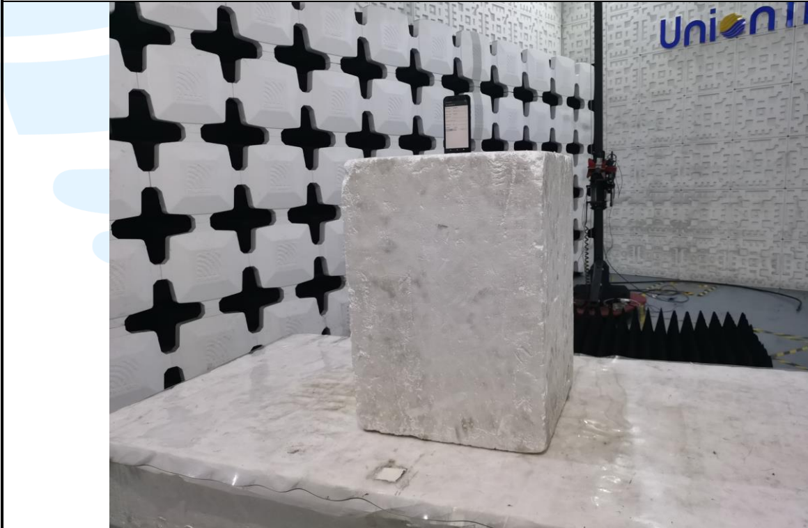
Radiated emission Test Setup (Above 1 GHz)
