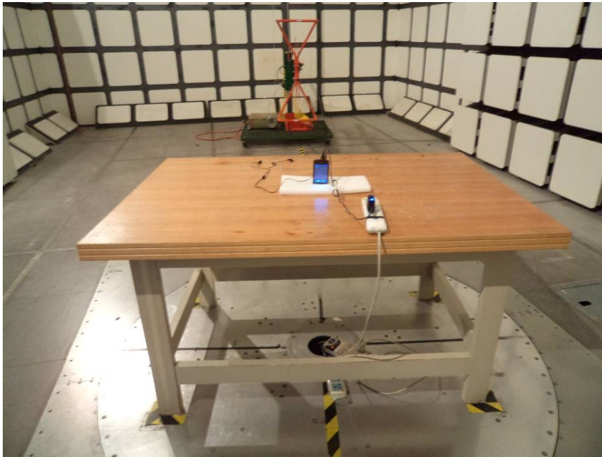
Radiated Emissions View (Below 1 GHz)
