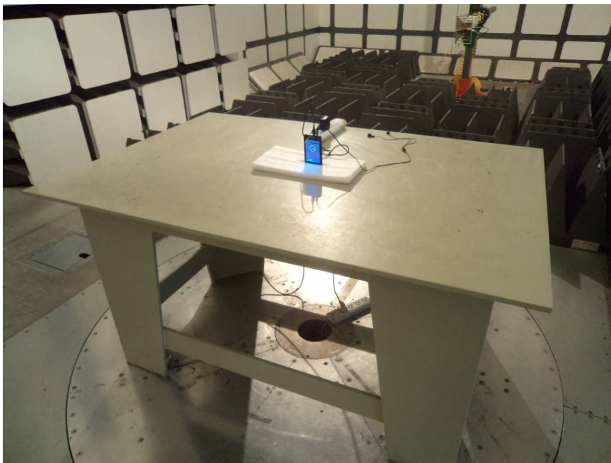
Radiated Emissions View (Above 1 GHz)
