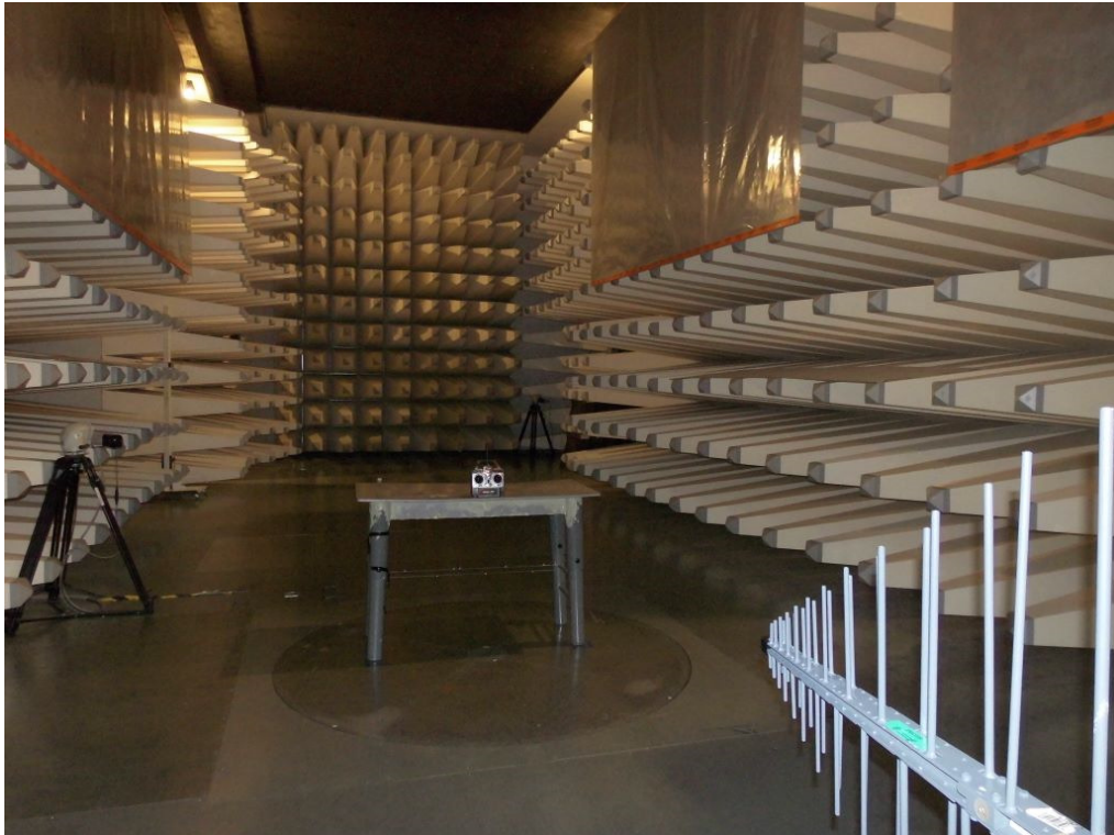
Setup for radiated emission
