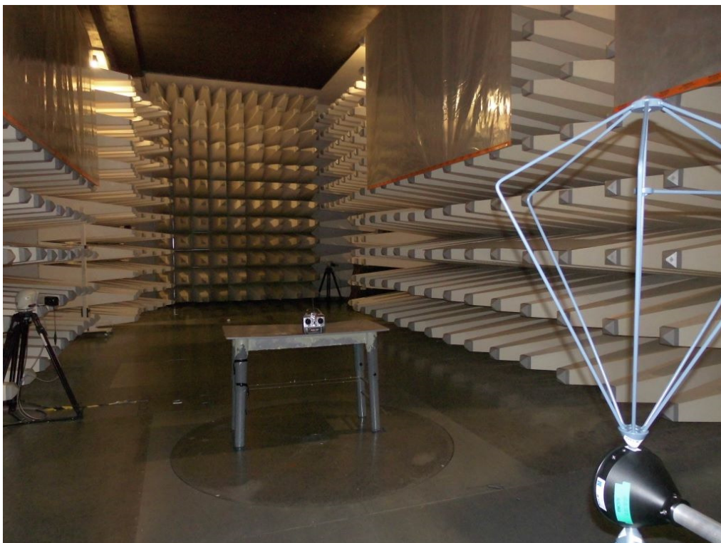
Setup for radiated emission
