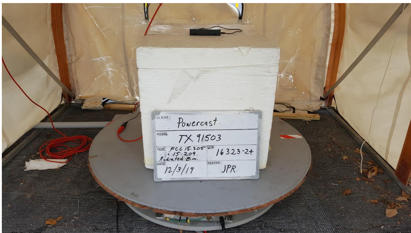
Photograph 2: Radiated Emissions Test Configuration – Flat
