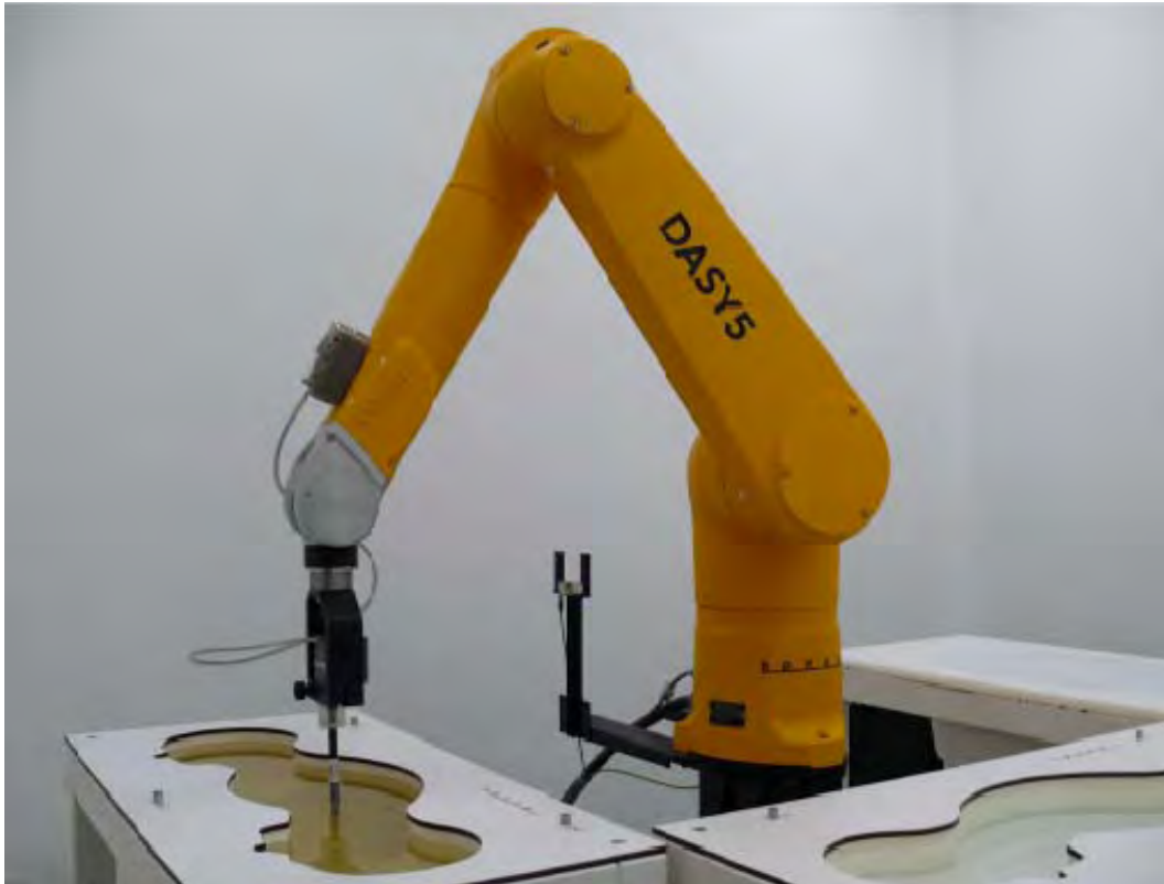
Picture 1: Specific Absorption Rate Test Layout
