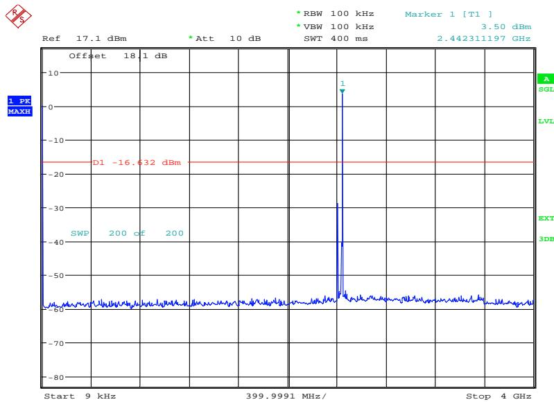
The plot above shows a second signal at 2402 MHz which is generated from the Bluetooth Test Set.
