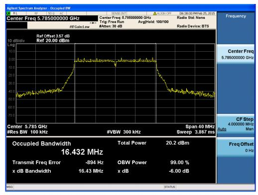
6 dB Bandwidth Test Mode: 802.11a & Ch.165 & ANT 2
