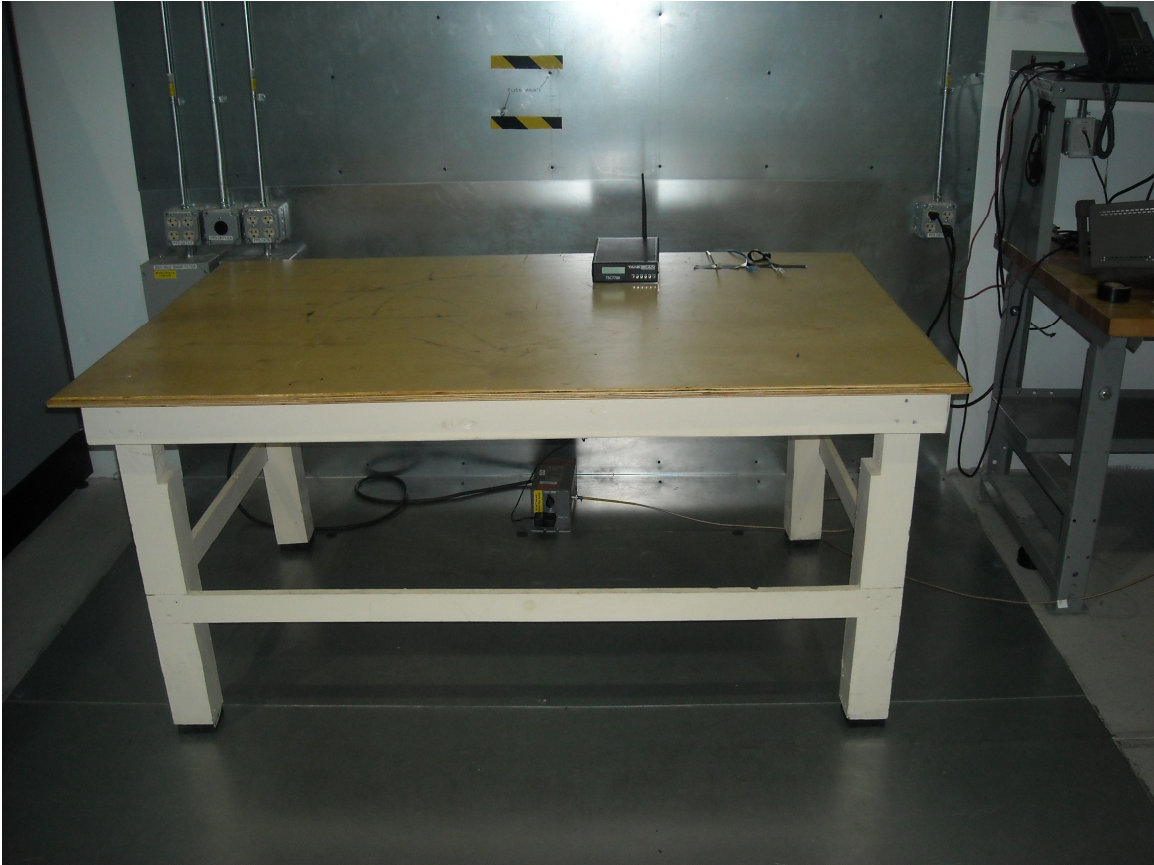
AC mains Line Conducted Measurements - Front
