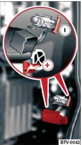
Fig. 247 Engine compartment: Terminals for jump leads and battery charger
