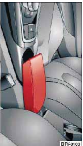
Fig. 55 Armrest between driver's seat and front passenger's seat
