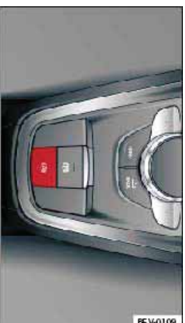
Fig. 79 Section of centre console: Button for hold assist
