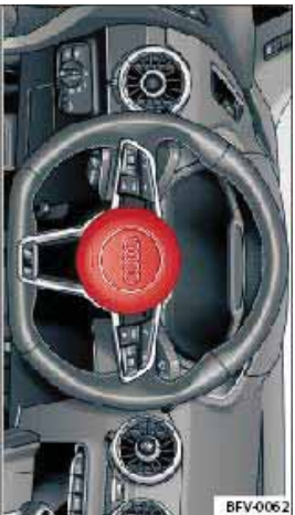
Fig. 206 Driver's airbag in steering wheel
