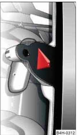
Fig. 15 Windscreen: Camera window for traffic sign recognition
