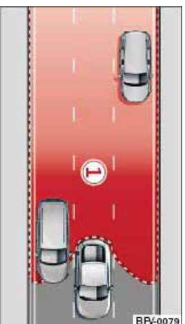
Fig. 99 Area covered by the radar sensors
