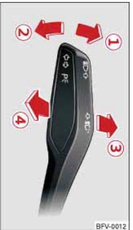
Fig. 40 Turn signal and main beam headlight lever
