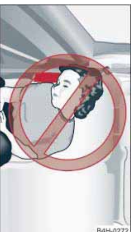
Fig. 1.83 Illustration of a dangerous sitting position near the opening for the side airbag
