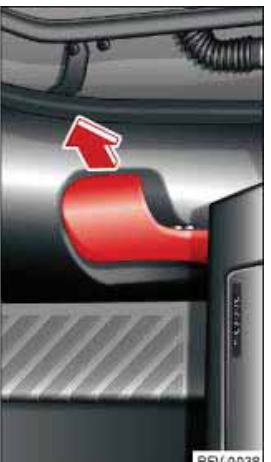
Fig. 219 Footwell on driver's side: Release lever
