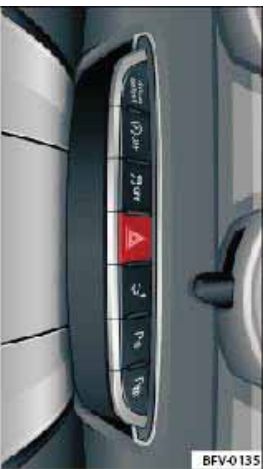
Fig. 42 Centre console: Switch for hazard warning lights
