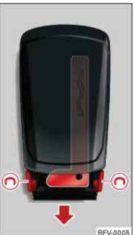
Fig. 25 Remote control key (rear): Removing battery carrier
