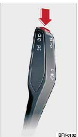
Fig. 95 Turn signal lever: Button for active lane assist
