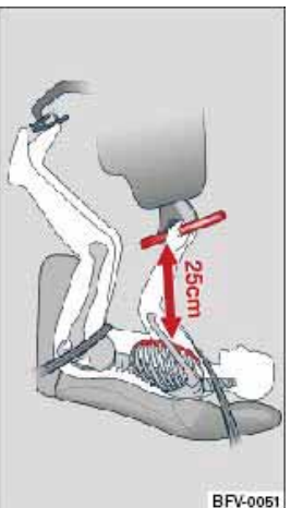
Fig. 182 Adjust seat and sit in correct position
