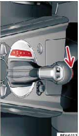
Fig. 82 Detail of the centre console: Selector lever with interlock button
