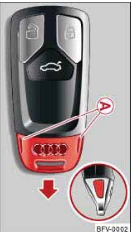
Fig. 22 Remote control key (front): Removing cap
