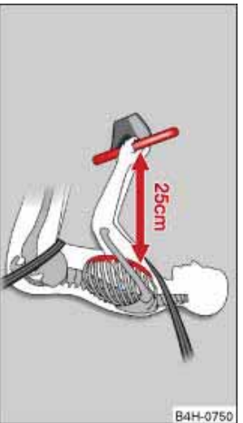
Fig. 209 Minimum distance from steering wheel
