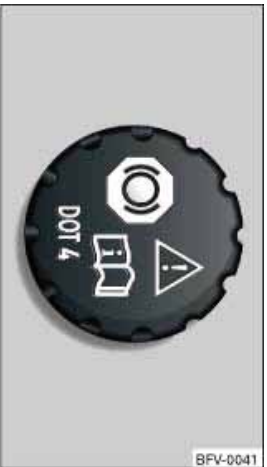
Fig. 225 Engine compartment: Cap of brake fluid reservoir
