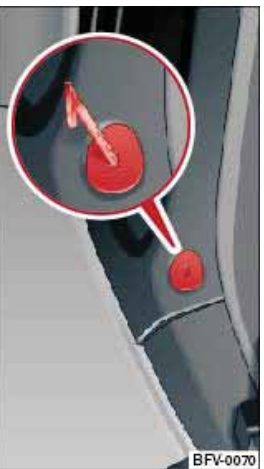
Fig. 33 Accessing manual release lever on left of luggage compartment below rear window
