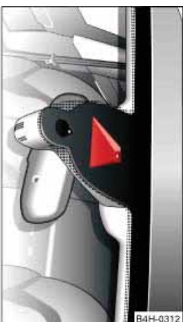
Fig. 96 Windscreen: Camera window for active lane assist
