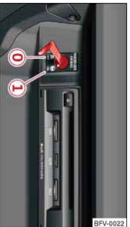
Fig. 204 Glove box: Key-operated switch for deactivating front passenger's airbag
