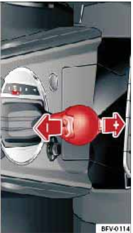
Fig. 83 Centre console: Manual gear selection using selector lever
