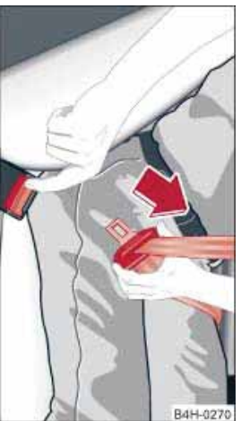
Fig. 202 The latch plate of the belt springs out of the buckle
