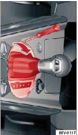
Fig. 87 Selector lever: Removing the cover
