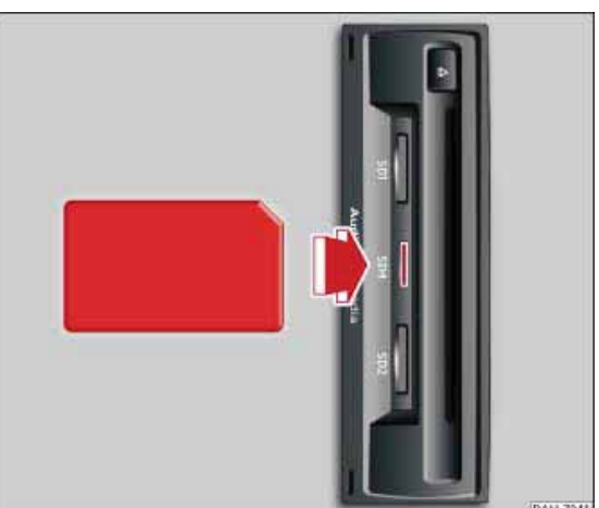
Fig. 136 Inserting the SIM card (mini SIM card, actual size)
