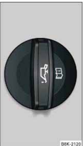
Fig- 223 Engine compartment: Engine oil filler cap
