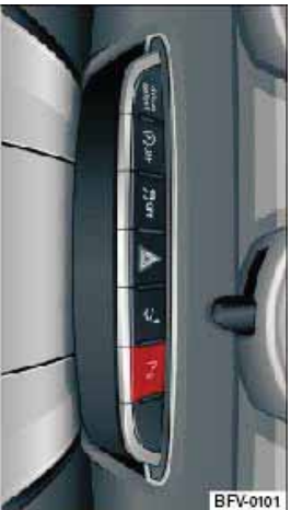
Fig. 106 Centre console: Button for parking aid
