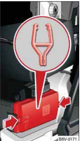
Fig. 255 Engine compartment, left-hand side: Fuse cover
