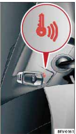
Fig. 74 Steering column/remote control key: Starting the engine after a malfunction
