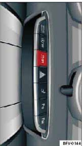
Fig. 115 Centre console (top): ESC button
