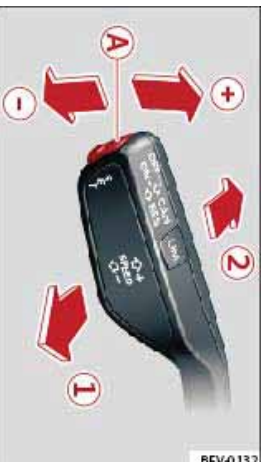
Fig. 89 Control lever for cruise control system
