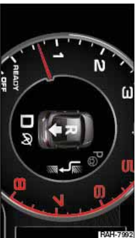
Fig. 113 Instrument cluster: Prompt to select reverse gear
