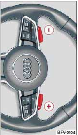
Fig. 84 Steering wheel: Manual gear selection with paddle levers*
