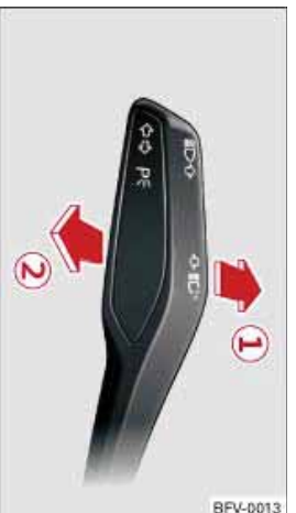
Fig. 41 Turn signal and main beam lever: Switching main beam assist on/off
