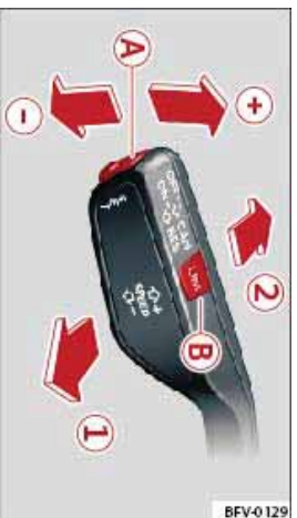
Fig. 93 Control lever for cruise control system
