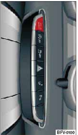
Fig. 103 Centre console: Button for drive select
