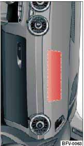
Fig. 207 Front passenger's airbag in dashboard
