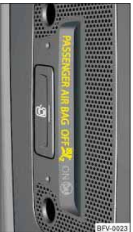
Fig. 205 Headliner: Warning lamp lights up when passenger's airbag is deactivated
