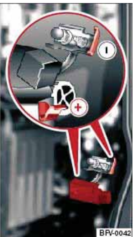
Fig. 226 Engine compartment: Terminals for jump leads and battery charger
