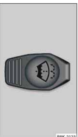
Fig. 227 Engine compartment: Cap of windscreen washer container
