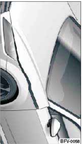
Fig. 191 Bonnet: Pedestrian protection system triggered
