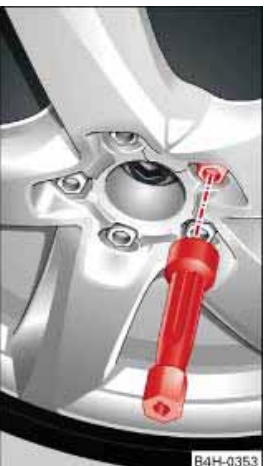
Fig. 243 Wheel: Hexagonal socket for turning wheel bolts
