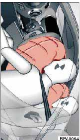
Fig. 208 Front airbags in inflated condition
