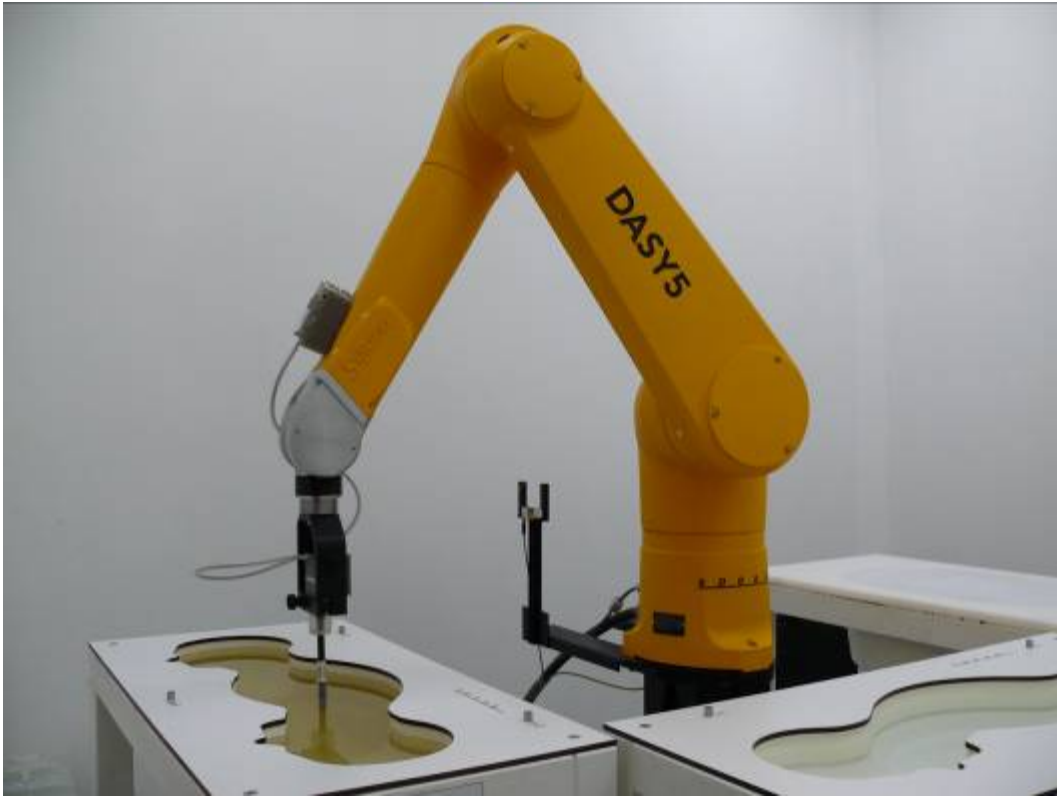
Picture 1: Specific Absorption Rate Test Layout
