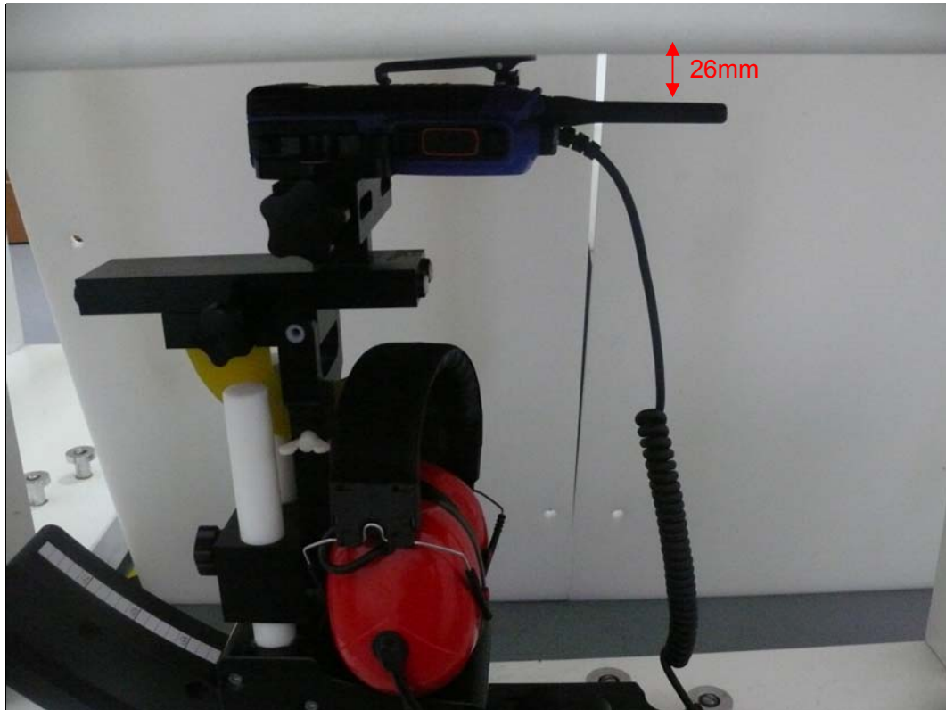
Picture 6: Body-worn with Speaker-Microphone, the front of the EUT towards ground, Belt clip attach the Phantom, the distance from EUT Antenna to the bottom of the Phantom is 26mm
