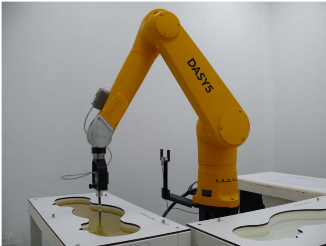
Picture 1: Specific Absorption Rate Test Layout
