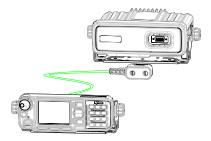
**Step 4** Connect the accessories following Step 4 for installation of mobile terminal.
