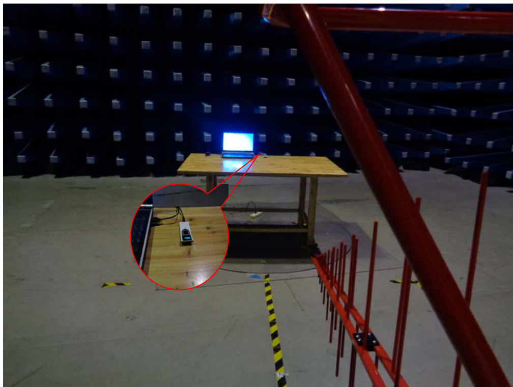
Radiated Emissions Setup Below 1GHz Front View
