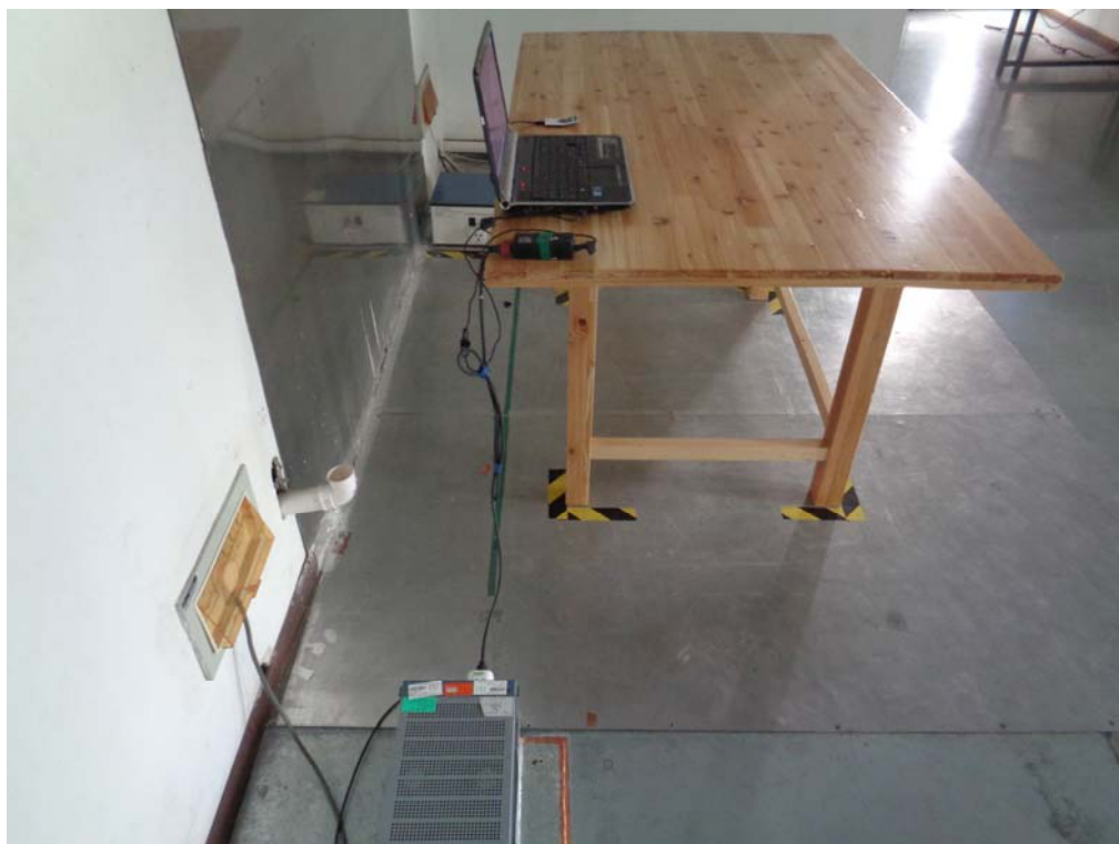
Conducted Emissions Setup Side View
