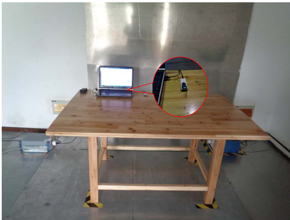
Conducted Emissions Setup Front View
