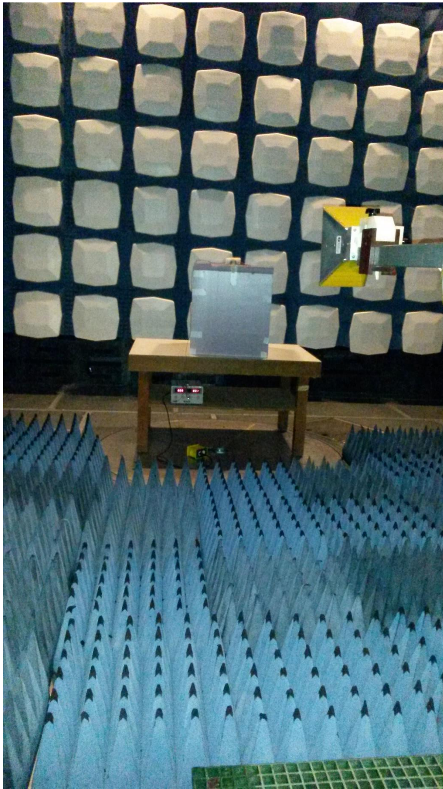
Radiated Emissions Setup in Semi-Anechoic Chamber, Above 1GHz
