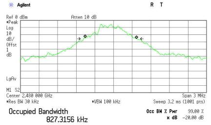
Transmit Freq Error -43.008 kHz х dB Bandwidth 865.387 kHz
