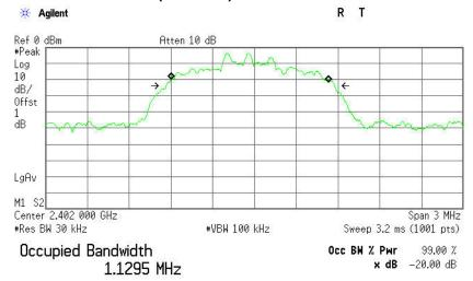
Transmit Freq Error -32.880 kHz x dB Bandwidth 1.210 MHz
