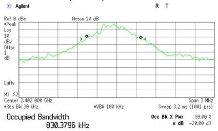
Transmit Freq Error -41.940 kHz x dB Bandwidth 858.178 kHz
