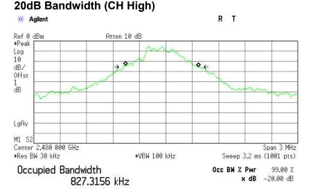
Transmit Freq Error -43.008 kHz x dB Bandwidth 865.387 kHz
