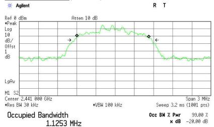
Transmit Freq Error -35.526 kHz x dB Bandwidth 1.211 MHz
