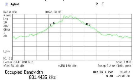
Transmit Freq Error -42.820 kHz x dB Bandwidth 864.207 kHz
