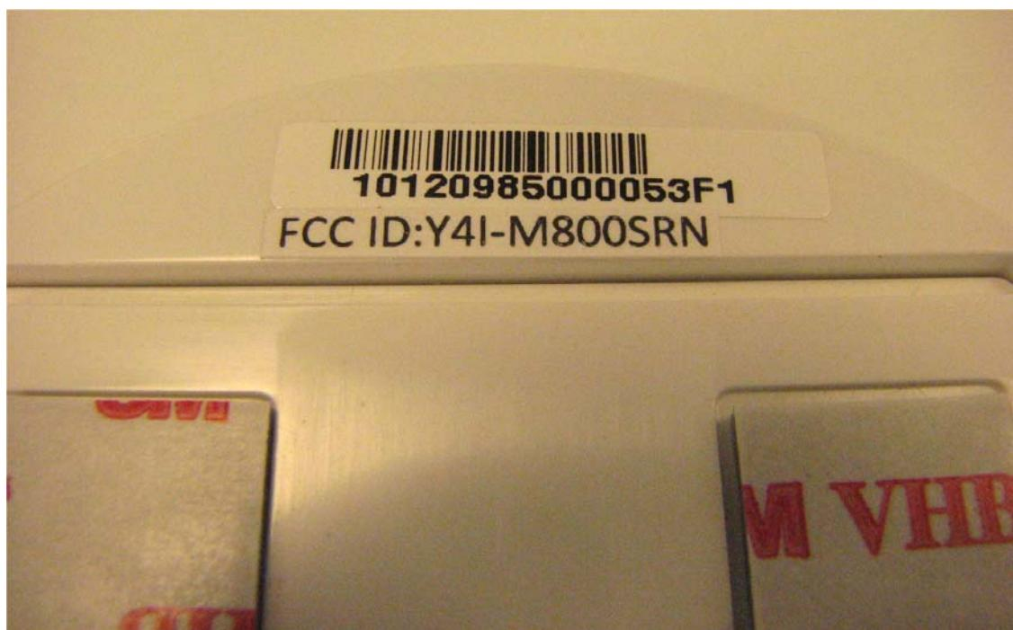
Label with **FCC ID:Y4I-M800SRN** is located at the rear side panel. The statement according to FCC part 15 §15.19(a)(3) is placed in User's Guide (Application exhibit User\_manual\_23372).
