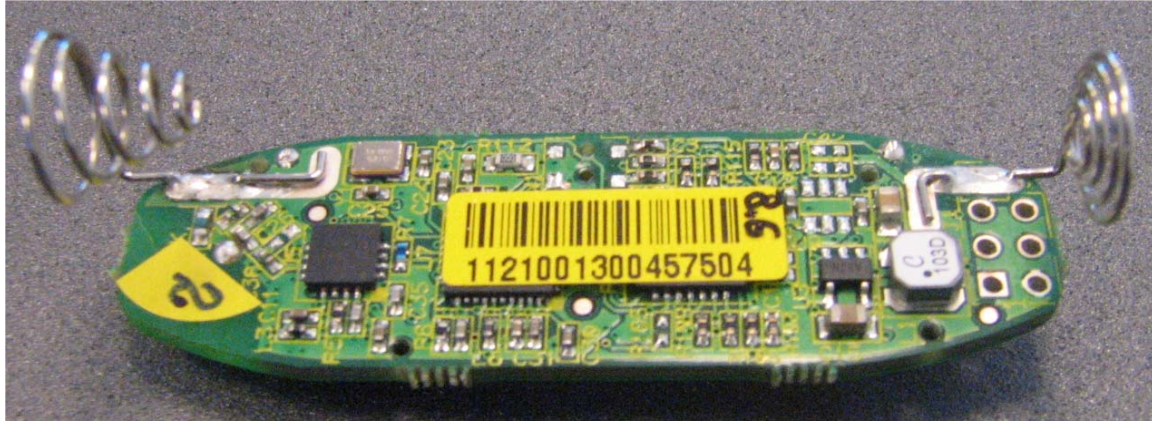
Photograph No.6 M800MGL magnet sensor (detector) PCB second side view
