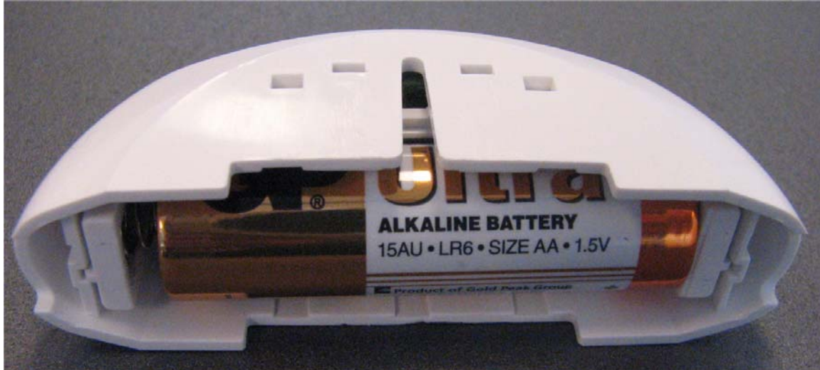
Photograph No.2 M800MGL magnet sensor (detector) view with battery
