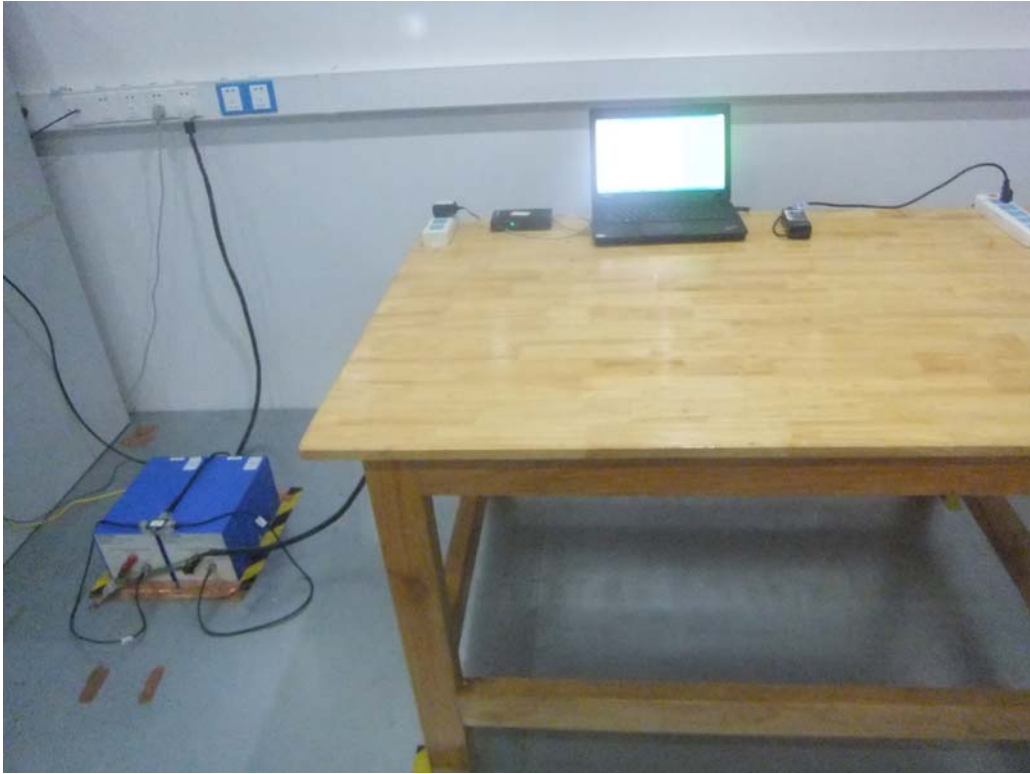
Conducted Emissions Test Setup Front View
