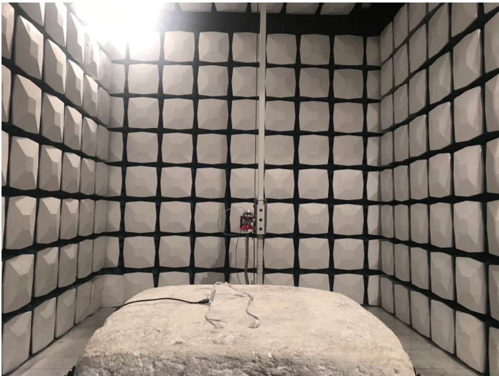
Description: Radiated Emission Test Setup for 1~18GHz
