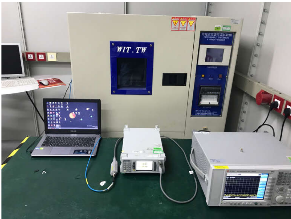
Description: Conducted Test Setup
