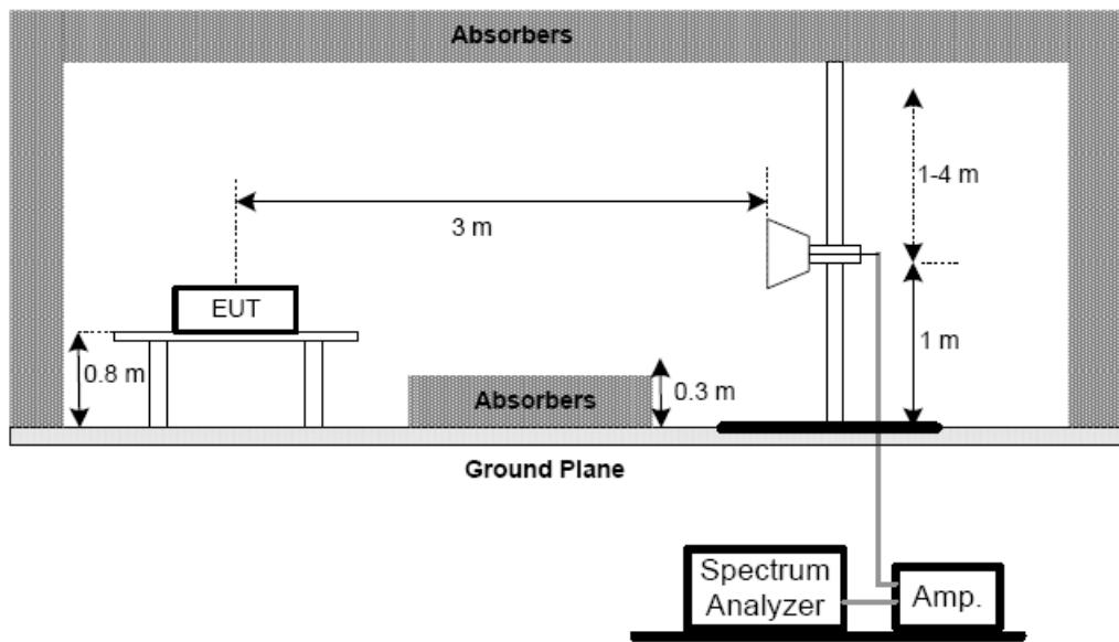
(C) For radiated emissions below 30MHz
