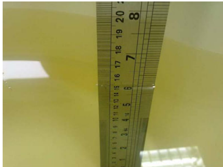
Liquid depth in the Flat Phantom (1900MHz-Body)
