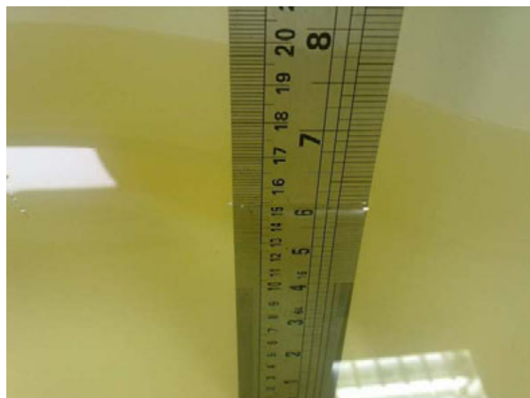
Liquid depth in the Flat Phantom (2450MHz-Body)
