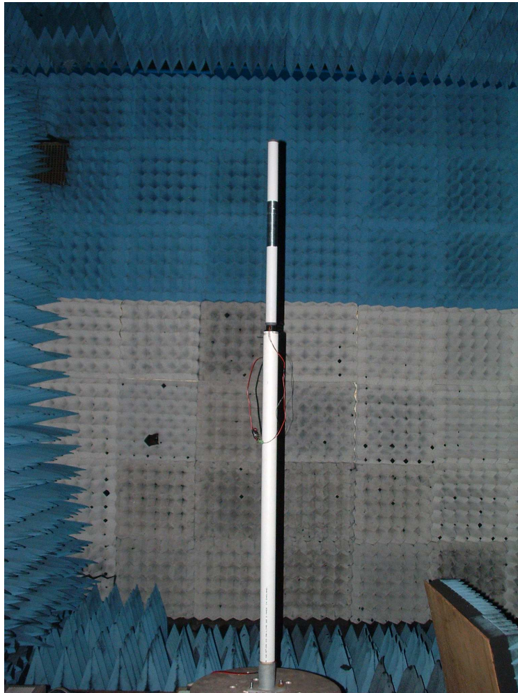
Figure 1 ACTIVE-XS dual band RTE mounted in the anechoic chamber
