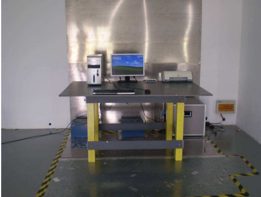
Conducted Emission Set-up Front View
