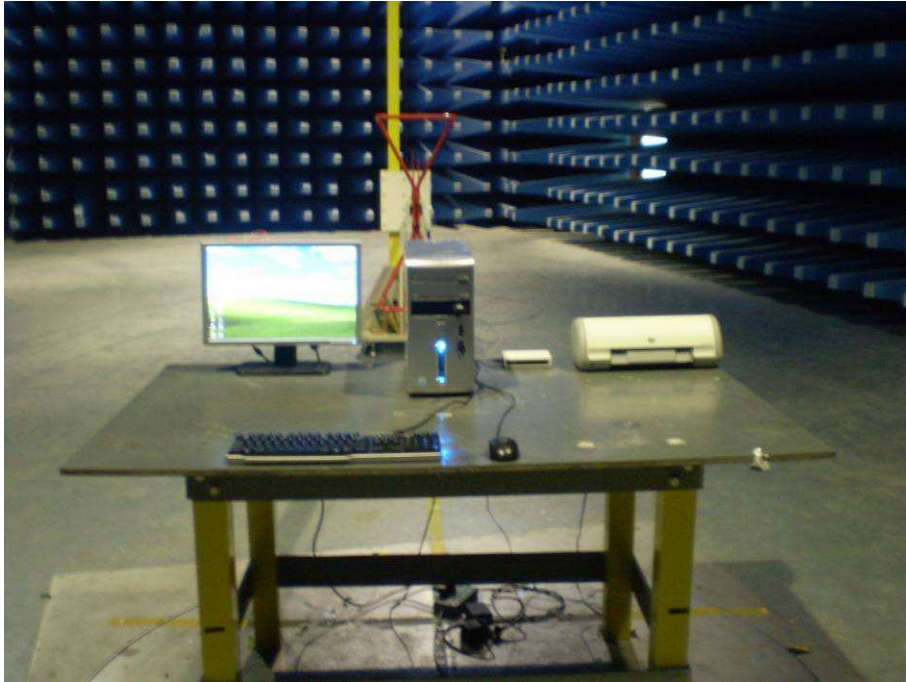
Radiated Emission Set-up Front View
