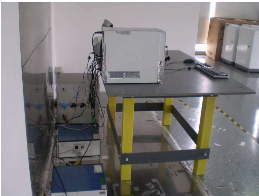
Conducted Emission Set-up Side View
